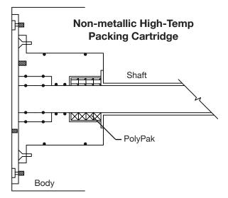
**Packing:** Valves shall incorporate cartridge style live loaded self-adjusting packing that is field replaceable without removal or disassembly of the valve from the piping for the application. Packing shall consist of minimum 3 rings of 0.25" Grafoil in each journal. Dual packing will be used as required with external bearings. The cartridge shall be field replaceable without removal of the valve from the pipe. Poly-Pak retention shall be retained by a shoulder as part of the cartridge.
