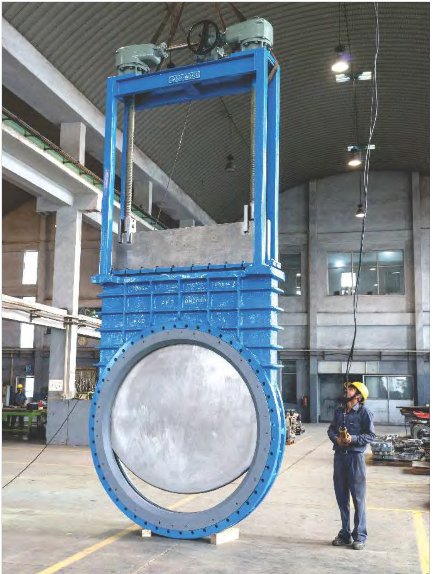
DN 2000, Bi-directional, PN 10 rated bonnetless tandem spindle electrically operated knife gate valve
