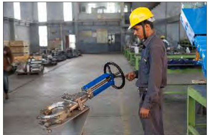
Very low operating torque compared to conventional knife gate valves
