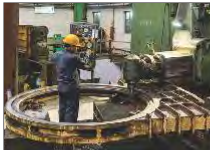
Large floor boring machine
